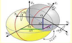
**Conversion** changes coordinates remaining the same datum (e.g., ellipsoid axes). Conversion example: mapping of ellipsoidal to Cartesian coordinates using a map projection
